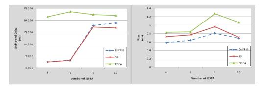
Fig. 7 – End-to-end delay vs. number of QSTAs
